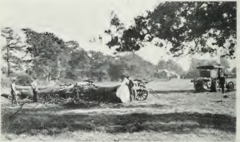
FIG. 46. LOADING LOGS ON TIMBER WAGON. [By courtesy of "Sentinel" Waggon Works, Ltd.]
